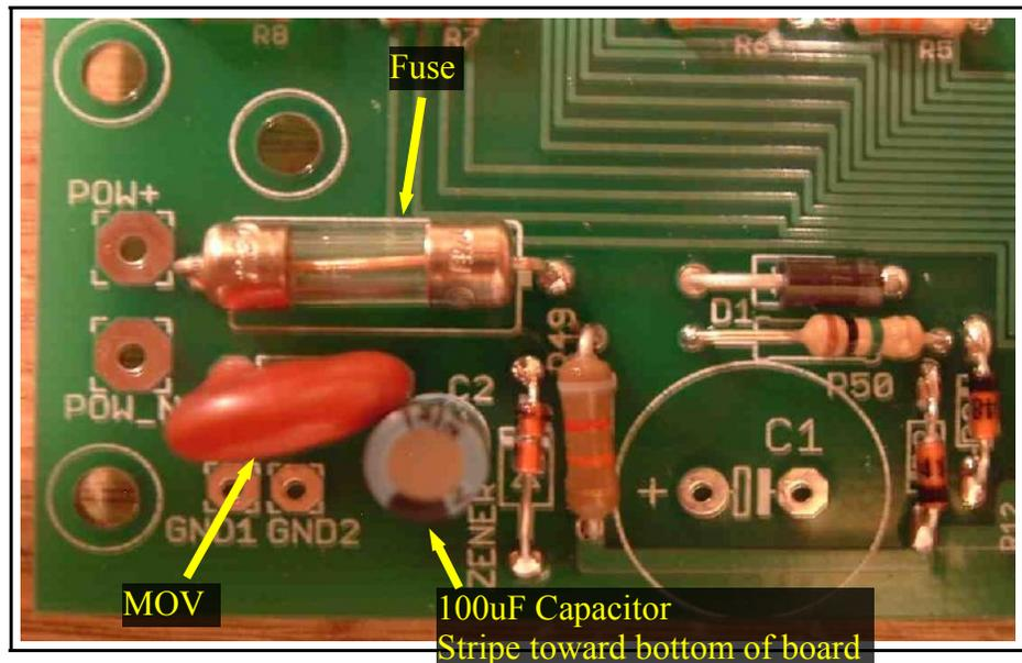
26) Solder the MOV in place. Orientation does not matter. Snip off the extra lead wire on the back.
