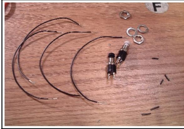
32) Cut the wire into 4 pieces, each about 4 inches long. Strip about 1/4" from the ends of each piece of wire.
