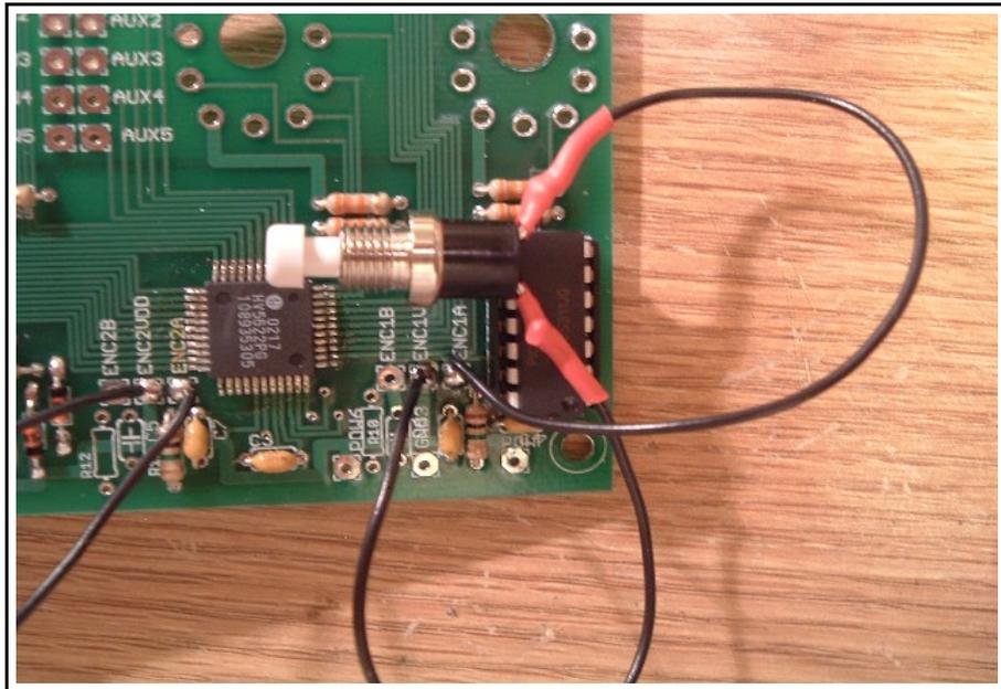
36) Solder the 2 open ends of the wires for the white button into ENC1VDD and ENC1A.
