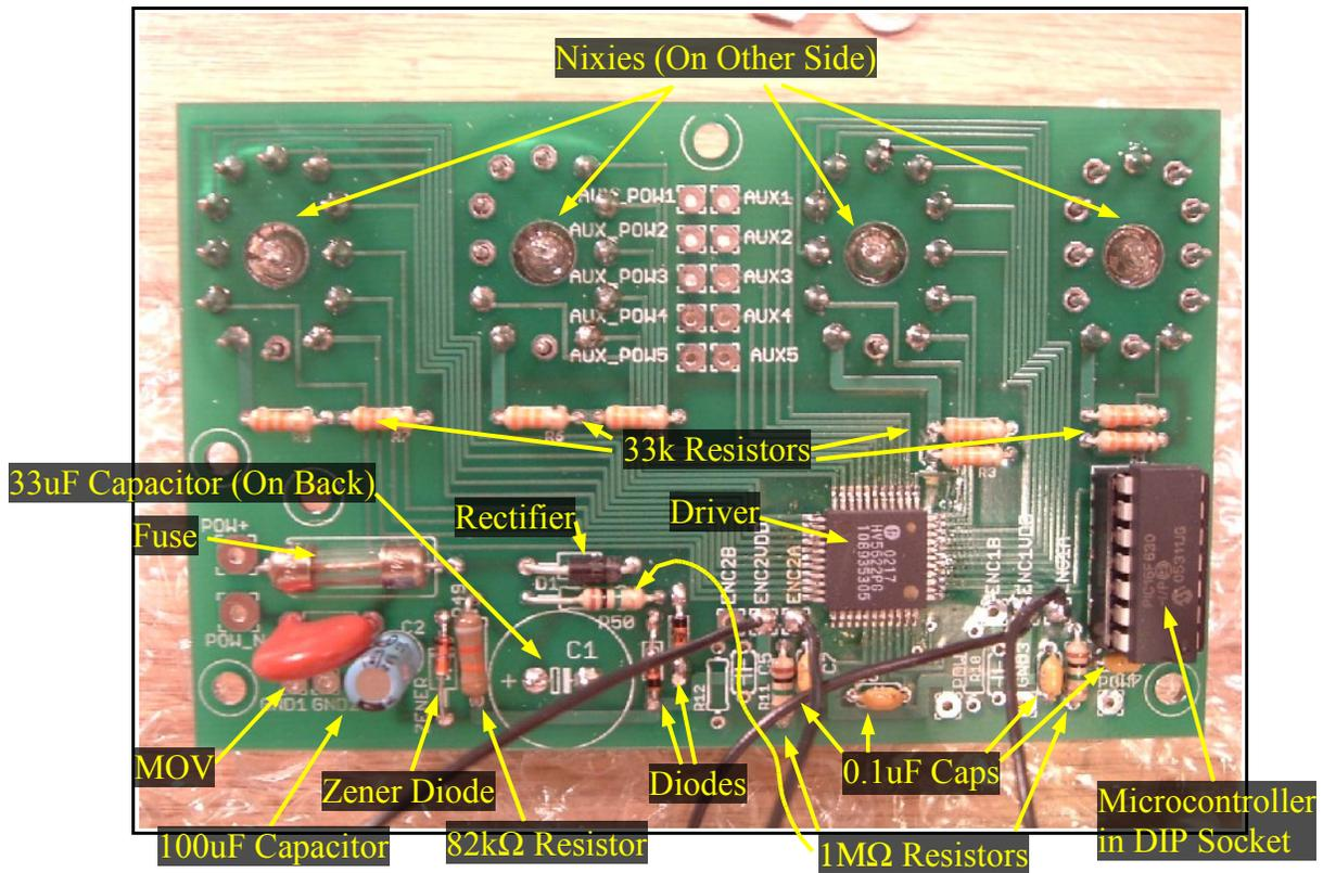
**Update:** The board now has a place for an extra capacitor (C9) across the signal diodes. This is not pictured above. The new additional capacitor C9 goes above the Rectifier, and the Rectifier has been moved slightly up and to the left. Please see step 30.
