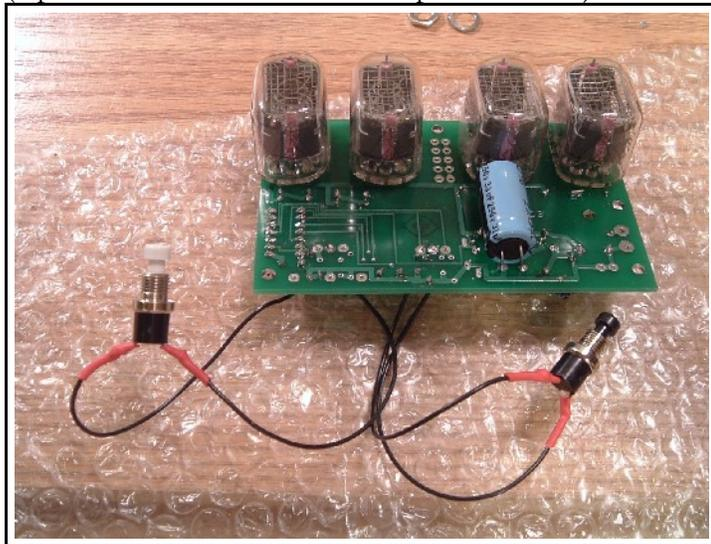
39) Turn the board over, holding the Nixies in Place, and solder 1 pin on each Nixie. The Nixies should now stay in place as you turn the board over, and check that the Nixies are resting flat against the board. If they are not, hold a hot soldering iron against the pin that was soldered, and press the Nixie flat against the board. When the solder melts, it will allow the Nixie to move; when the iron is removed, the solder will harden and keep the Nixie in position.
