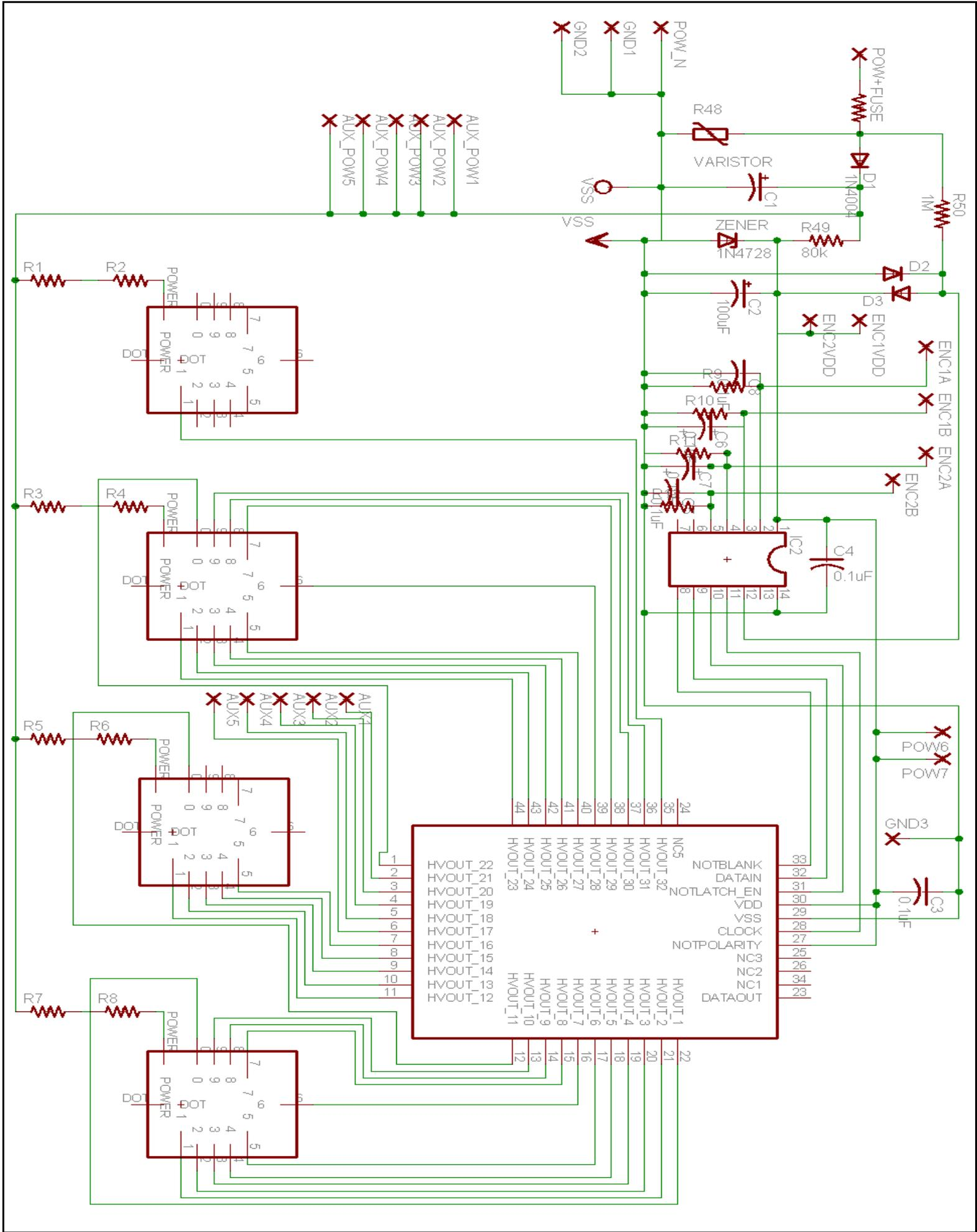
The low voltage supply is provided by a resistor and a Zener diode acting as a voltage divider. The ½ watt 82k Ohm resistor (R49) limits the current flow, and the Zener keeps the voltage at about 5V DC. A 100uF capacitor (C2) across the Zener filters the 5V power supply, keeping it stiff, and allowing the clock to go without power for 5 to 10 seconds without losing the time.
