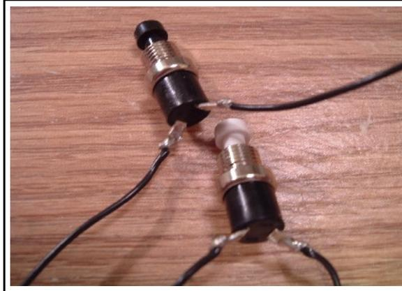
34) Slide a short piece of heat shrink over each wire and button lead, and shrink in place with heat gun or hair dryer. If a heat gun or hair dryer is not available, the heat shrink can be shrunk with careful use of the soldering iron, placed close
