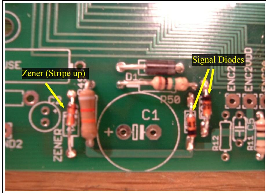
22) Solder signal diode D3 in its spot, with the stripe toward the BOTTOM of the board. This is the left hand diode, and the stripe goes towards the bottom of the board. Snip off the extra lead wire on the back.
