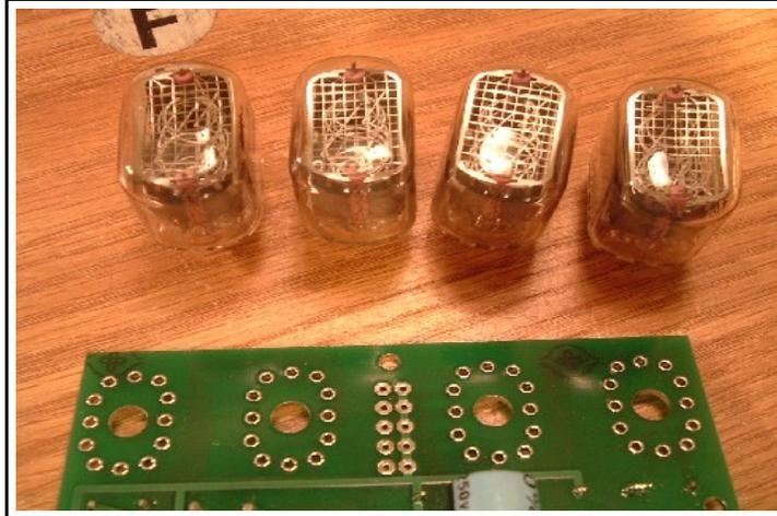
38) Place the 4 Nixie tubes into the mounting holes on the back of the board (the side with the physically larger 33uF Capacitor). **ORIENTATION MATTERS.** There is an arrow on the glass pointing to pin 1, which should be towards the bottom of the PCB when placed. To check alignment when the Nixie is in place, look for the number “3” and “4” filaments in the Nixies, and make sure they are right-side-up (top of the numbers towards the top of the board).
